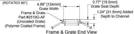
See Above for Actual 6.1" [155mm]-**Grate Selection** 3.94" [100mm] Independently Anchored Frame Anchor Bolt-Concrete Slab Depth Varies **Expansion Joint Both** Sides (Recommended) Lock Insert Monolithic Pour Lock Down Device 4" [102mm] Minimum All Sides Anchor Rib **Precast Polymer Concrete** Trench Drain Part #PD04 Soil Subgrade **End Cross Section View**
